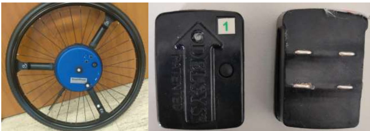
Figure 9: SmartWheel (left) and EMG device of Delsys with surface electrodes (right).
