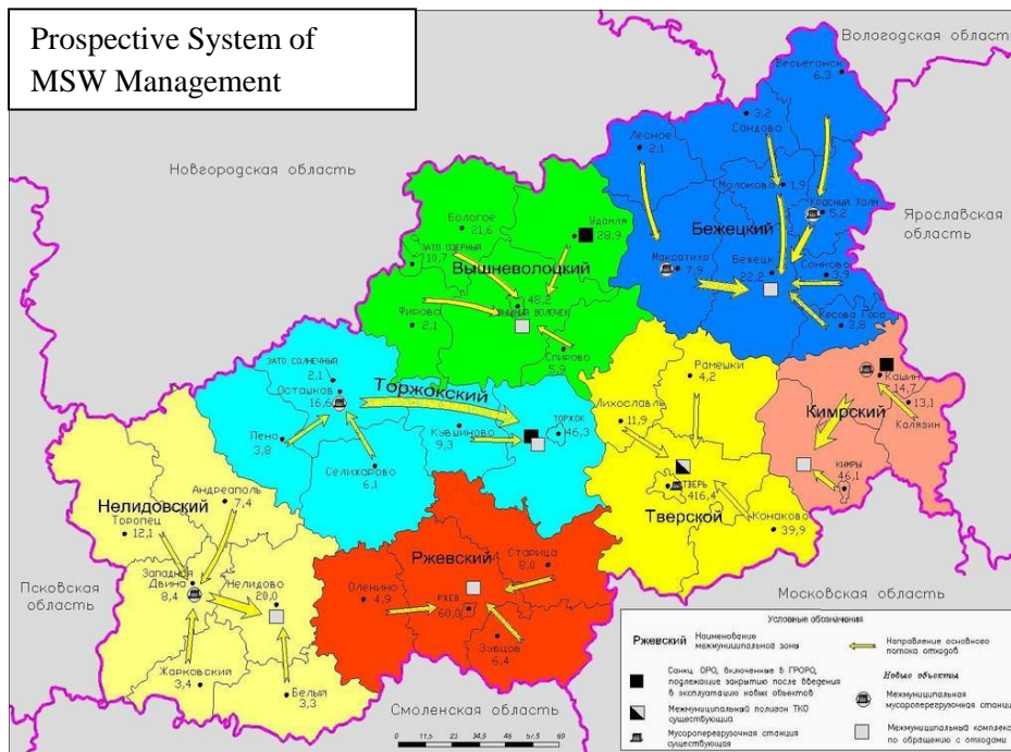
Figure 9. Example TS of Tver region: MSW flows from generation to treatment facilities (TS Project in Tver Region, 2015).
