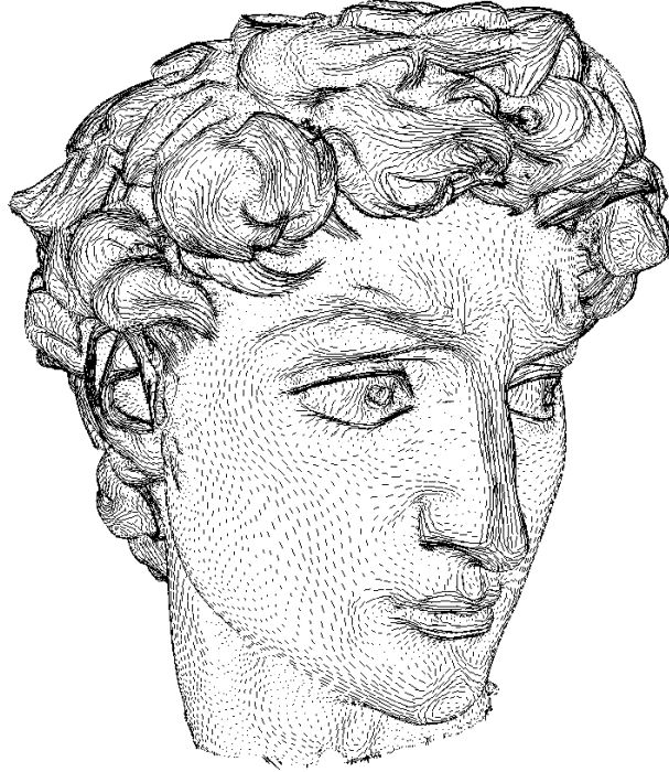
Figure 2.8: Minimal curvature directions estimated on a mesh of Michelangelo's David, based on definition 2.30. Image from [8].
