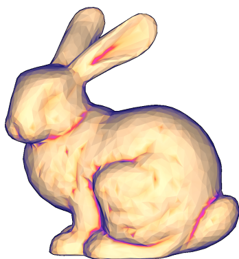
Figure 1.1: The model of a bunny. Large estimated curvatures of the surface are colored purple. http://graphics.stanford.edu/data/3Dscanrep/
