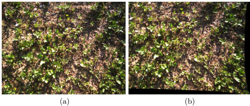
Figure 3.7: (a) Distorted image (b) Undistorted image
