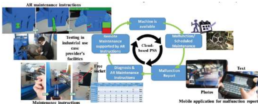
Figure 11: The framework of the sustainable Product Service System based on AR 142
