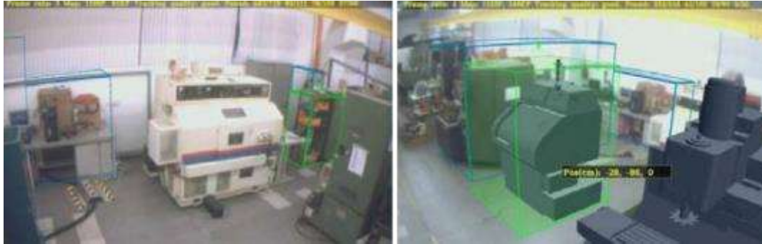
Figure 14: Layout planning for manufacturing facility to assist the on-site workers using AR. 155
