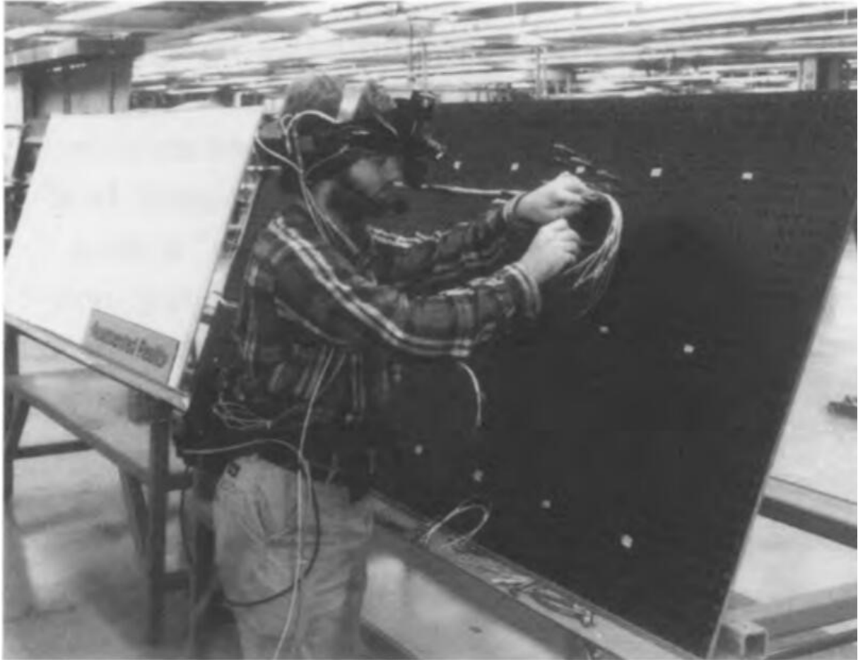
Figure 15: Adamjanin demonstrates Boeing's prototype wire bundle assembly application 176
