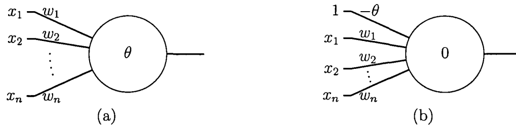
Figure 3.7: Perceptrons with stimulus threshold \theta (a) classical representation, and (b) equivalent representation with input vector in homogeneous coordinates
