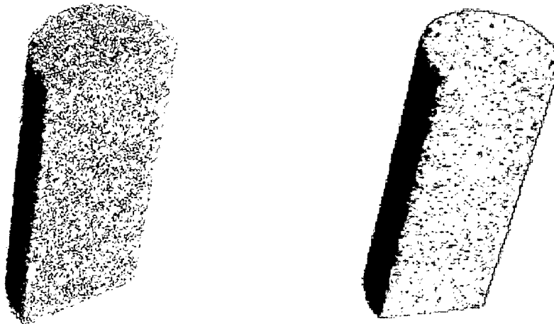
Fig. 7.16: 3D reconstructed images from 60 NT projections of a pure steel rod having 1.0 cm diameter (left image without smoothing and right image smoothing with median filter).
