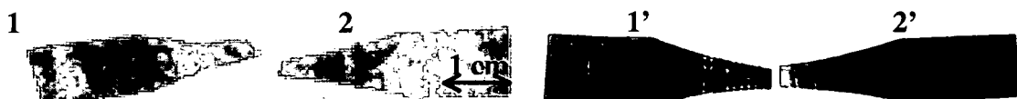
Fig. 5.26: Thermal NR (left images) and X – ray (right images) inspection of irradiated Alstom type R – glass fiber tapes (the samples 1 – 1' and 2 – 2' are the same ones).
