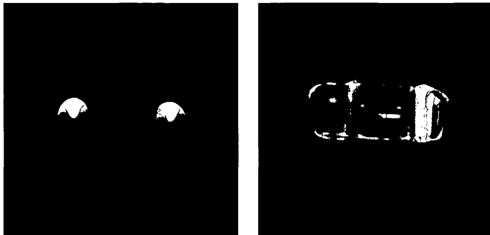
Fig. 4.10: Back projections of 55 th and 120 th slices at the position 1 and 2, when the rotation axis is not in the center.
