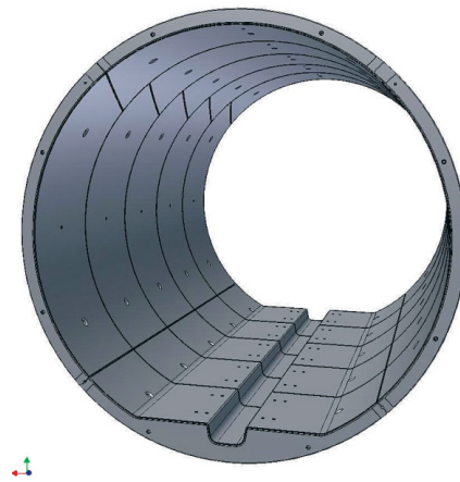
(b) Segmental lining system [26].
