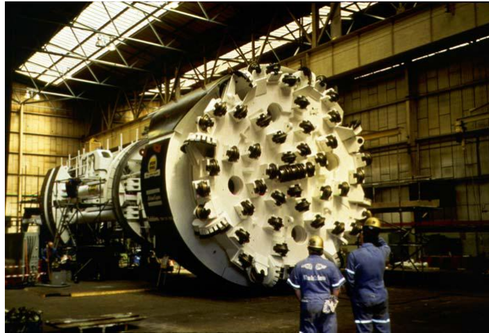
Figure 3.5: TBM for Queens water tunnel [31], [33].
