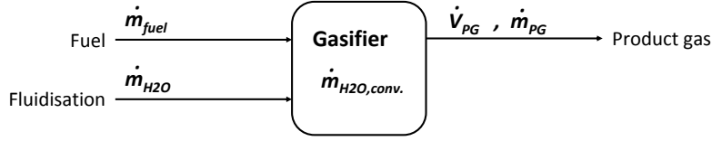
Figure 2.9: Global mass and species balance for the gasification reactor
