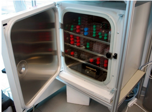
FIG 2.6: Incubator with CO 2 - and temperature-controlled atmosphere. The inner lining and racks are made of stainless steel. On the bottom a reservoir provides water for a humidified atmosphere and an external gas container is used as a CO 2 supply.
