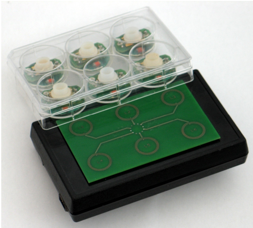
FIG 4.18: Realized system. The black box is the base station. The upper transparent part is a microtiter plate with the RFID-based tags with sensor devices attached on it. The dimensions of the base station are 145 \times 90 \times 30 \text{ mm}^3 .
