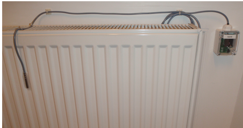
Figure 56. Sensor setup to measure the mean radiator temperature
