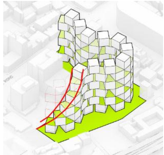
Figure 5.6: The volume is lowered at one side in order to break down the scale of the building ( http://www.big.dk/#projects )
