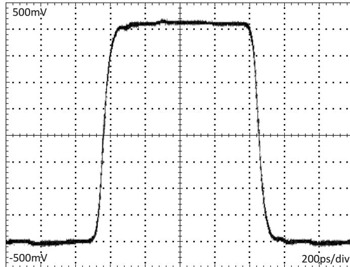
Figure 6.15: Transient response of 8-channel receiver with PIN7 photodiode @ 1 Gbps
