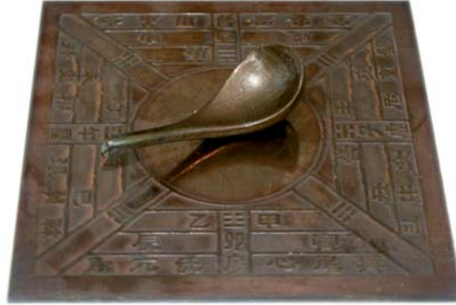
Figure 1.1: The device described in this figure is considered to be the earliest form of a magnetic compass [3].
