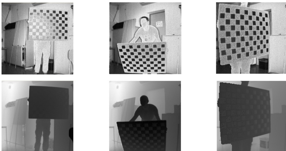
Figure 5.2: A sequence of intensity and depth images taken with the PMD[vision] Camcube 3.0
