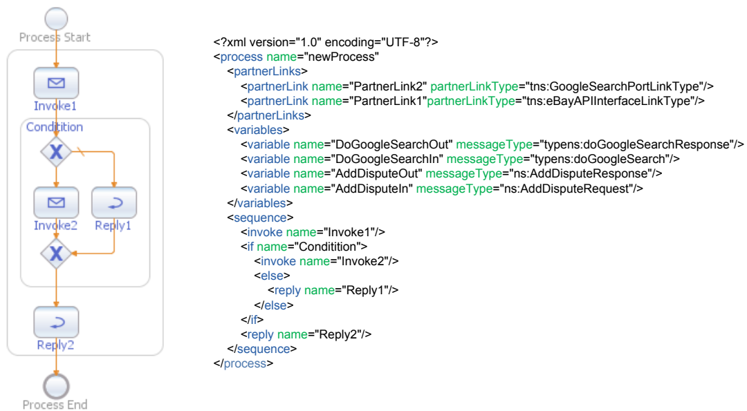
Figure 1.1.: Sample Workflow in BPEL Notation - Graphical and XML Representation
