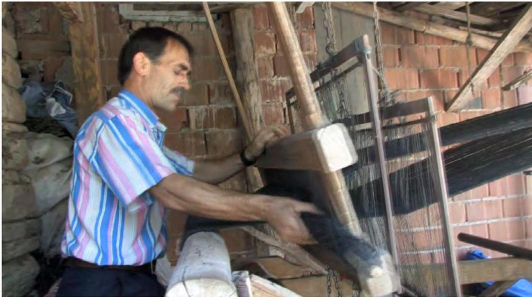
*image 4.092: The bobbin is driven through the shed.*
