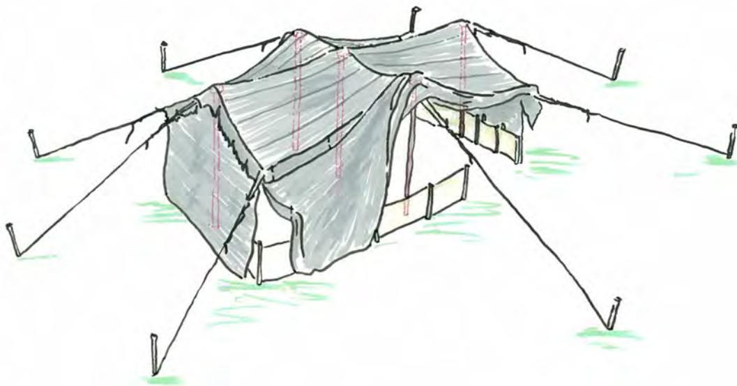
*image 2.004: Yörük five-pole tent of the Sarıkeçili. The miniature sketch is a simplified copy of the orthometric drawings presented by Böhmer<sup>172</sup>*
