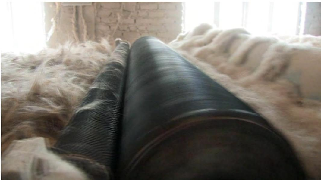
*image 4.066: The wool is driven forward by several fine-toothed rollers on which rows of fine needles take the fibres apart by swift left and right movements along the axis. There, the wool is spread out over the whole width of the machine and cleaned from foreign particles. This process can be compared to the manual beating with a bow.*
