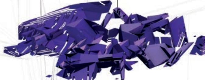
Inner shell{wall} out of fiber composite material extruded and grown on base of the wall support truss.
