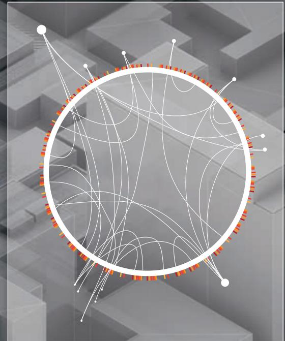
Predefining the optimal siting for the nucleus inside the host building. The field diagram shows the best direction for the nucleus to develop. Structural and static analysis of the building serve as foundation for this analysis. Weaker areas of the building means better areas to develop but they are also carry less load.
