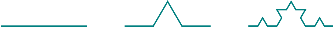
Figure 16: The first two iterations of the Koch curve. In each iteration the lines are divided into three equal parts. The middle part is duplicated and then arranged like a triangle.
