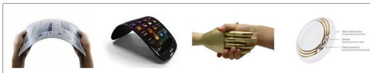
Figure 1: Organic electronic products based on OFETs from left to right: e-paper, 10 flexible display, 11 e-skin, 12 smart contact lens monitoring glucose level. 13
