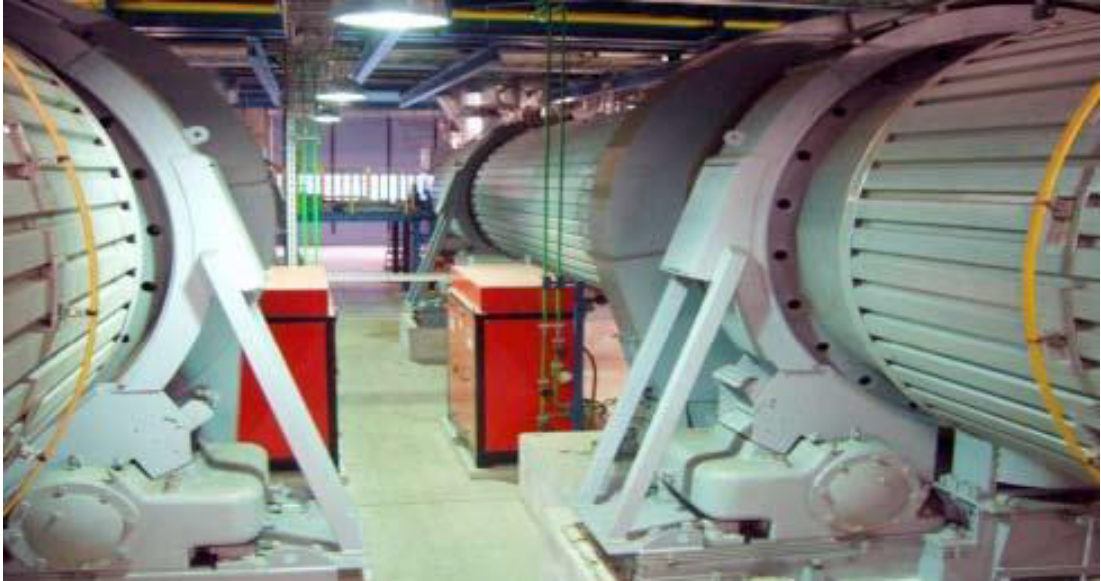
Figure 11: The picture above shows two of the conversion-drums. The drums are about 22 meters long, and 3 meters in diameter (source: own document)
