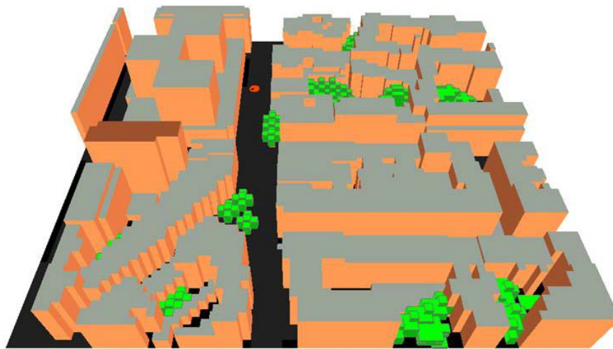
Figure 5-38: view of the 3D model after increasing the height of buildings up to 30% (scenario H2)
