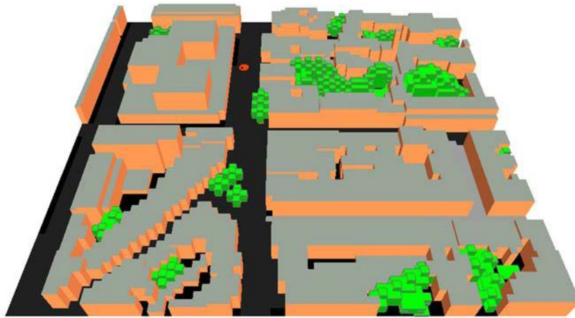
Figure 5-35: view of the 3D model after decreasing the height of buildings to 70% of their current condition (scenario H1)
