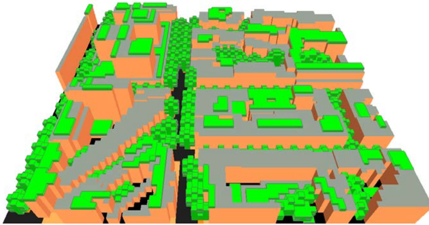
Figure 5-25: View of the 3D model after adding more trees and green roof as well as changing the sealing to the permeable pavement (scenario VM)
