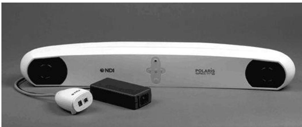
Figure 1.5: An actual optical tracker from NDI - the Polaris Spectra (MedicalExpo, 2015)
