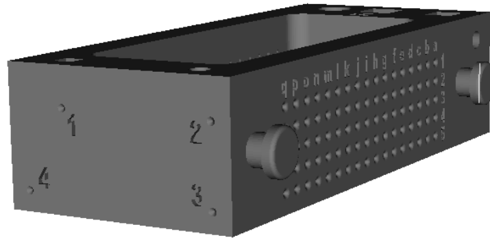
Figure 2.9: fCal phantom for calibration showing 4 of 8 landmarks
