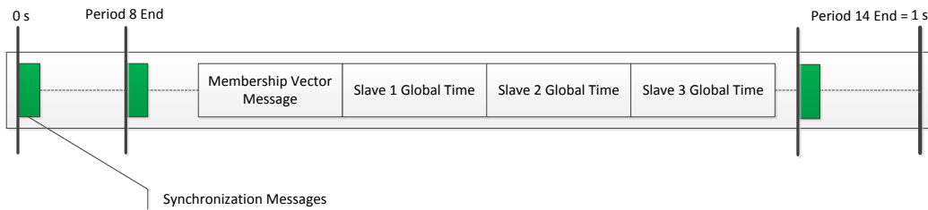
Figure 5.4: The relative placement of the messages required by the secure clock synchronization protocol in the application schedule.
