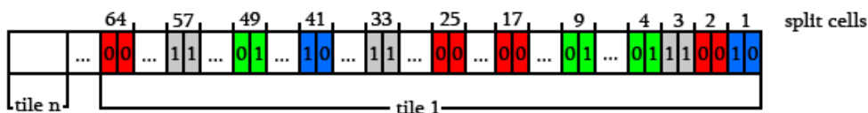
Figure 4.9: Bit allocation for the cell membership map. A tile is a 128-bit code containing 64 2-bit split cells. Each 2-bit code represents a split cell membership tag.
