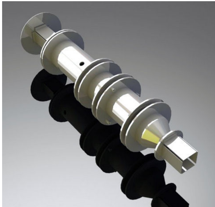
Figure 3.10: Computer model of the lens system used to focus and decelerate the ions when needed.
