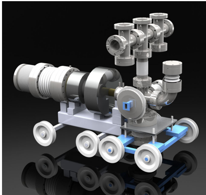
Figure 3.6: Computer model of the ion source SOPHIE at TU Wien used to produce the ions for the sputtering yield measurements
