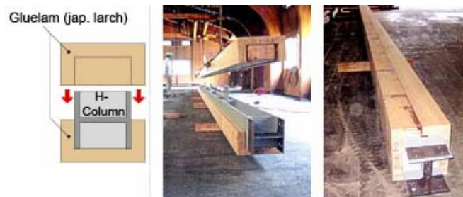
Fig 5.2.7.b – Hybrid construction explanation
