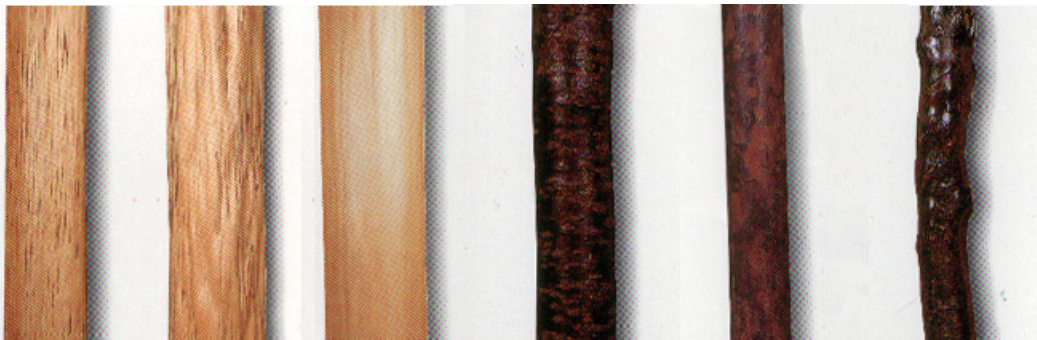
Fig 2.2.2.a – Examples for Tokobashira (from left to right: a) Kitayama cedar, three types; b) Japanese white birch; c) Japanese red pine; d) Plum;)
