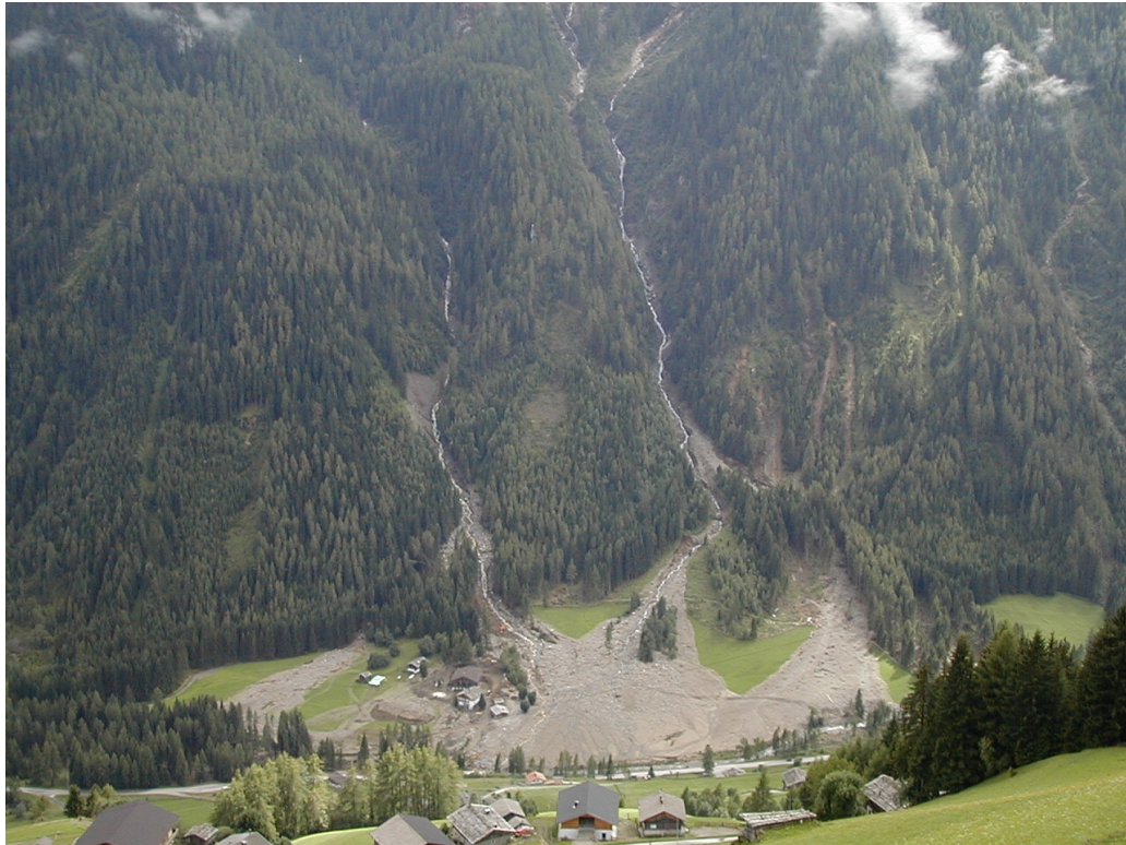
Figure 6.6 – Aerial view on the debris flow deposit from Abteilung30 (2010)
