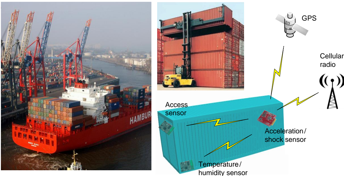
Figure 1.5: WSNs for container monitoring and tracking system: container port in Hamburg, and network topology for in-container observation system with external wireless communication link
