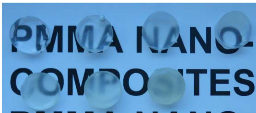
Figure 117. Photograph of in situ polymerized PMMA / MA-C10-TMS@SiO 2 nanocomposites, from left to right: upper row: blank matrix, 3 wt% and 5 wt% small SiO 2 , 10 wt % small SiO 2 , lower row: 3 wt%, 5 wt% and 10 wt % large SiO 2 nanoparticle content.
