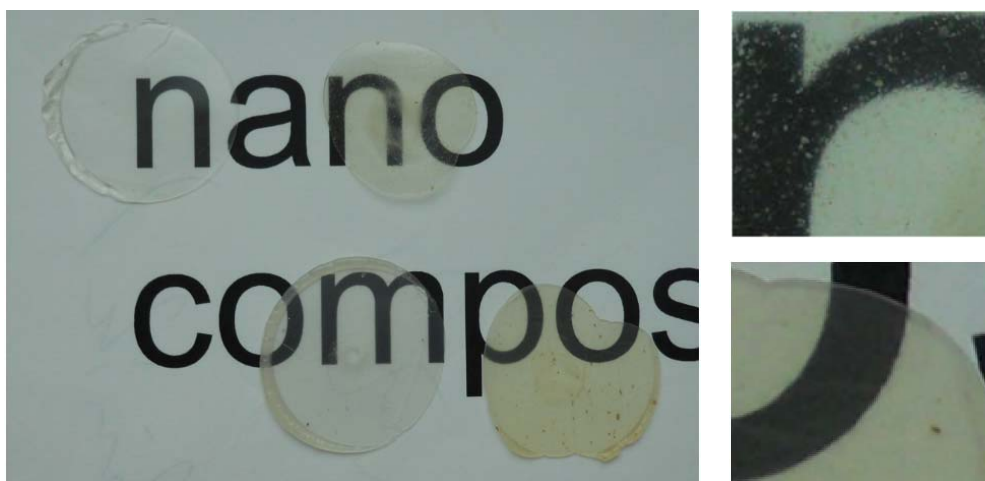
Figure 114. Photograph of extruded 5 wt% SiO 2 large nanoparticles with different surface modification in PS, prepared via melt-extrusion and compression molded to 0.25 mm plates. The overview picture shows, from left to right, in the upper row: blank PS (also extruded), unmodified SiO 2 (detail right upper picture), lower row: DTMS@SiO 2 , PS@SiO 2 (detail right lower picture).
