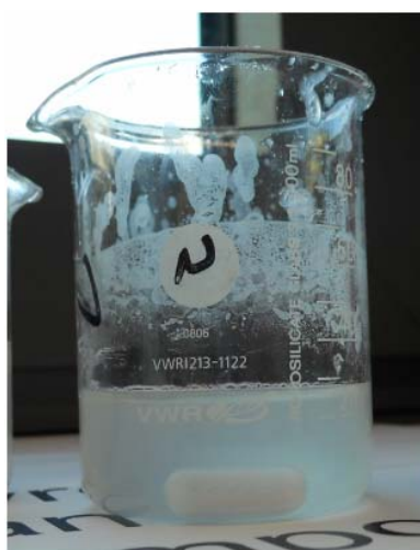
Figure 149. Photograph of solution compounded sample containing 5 wt% polystyrene shell \text{SiO}_2 large nanoparticles, before evaporation of the solvent.
