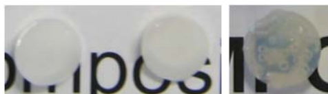
Figure 118. Photographs of in situ polymerized PMMA / ZrO 2 nanocomposites, left image: 3 wt% and 5 wt% large DPPA@ZrO 2 filler content, right image: 5 wt% MA-C10-PA@ZrO 2 (sample contains captured gas bubbles).
