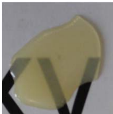
Figure 125. Photographs of nanocomposite plates containing (each 5 wt%) unmodified larger silica and zirconia nanoparticles leading to opaque materials as well as particles with appropriate surface modification leading to transparent materials.
