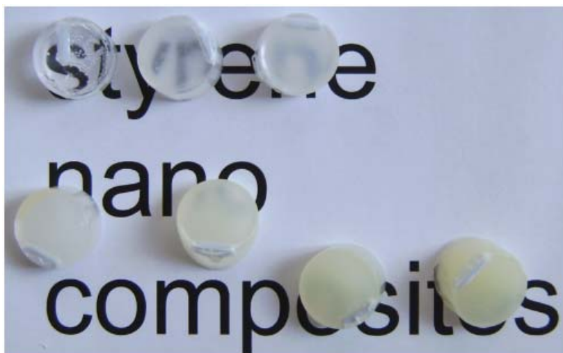
Figure 106. Photograph of in situ polymerized polystyrene \text{SiO}_2 (large, unmodified) nanocomposites, from left to right: upper row: blank matrix, 3 wt% and 5 wt% small \text{SiO}_2 , lower row: 10 wt % small \text{SiO}_2 , 3 wt%, 5 wt% and 10 wt % large \text{SiO}_2 nanoparticles content, captured stirring beads and some gas bubbles are also visible.
