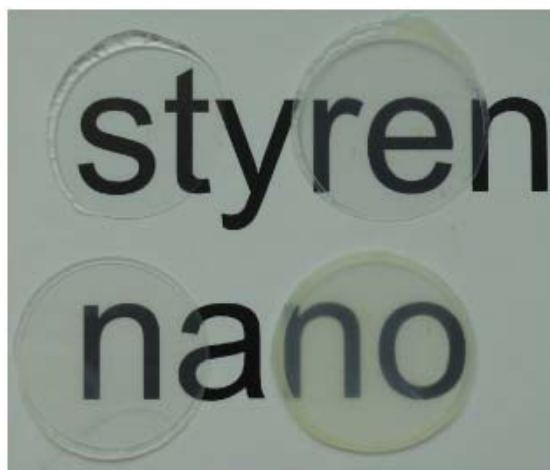
Figure 108. Photograph of compression molded, in situ polymerized, PS@SiO 2 large in PS. Plates with a thickness of 0.25 mm, from left to right: upper row: blank matrix, 3 wt% filler, lower row: 5 wt% filler, 10 wt% filler.
