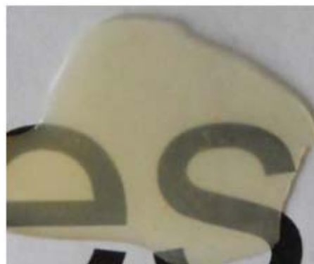
Figure 125. Photographs of nanocomposite plates containing (each 5 wt%) unmodified larger silica and zirconia nanoparticles leading to opaque materials as well as particles with appropriate surface modification leading to transparent materials.
