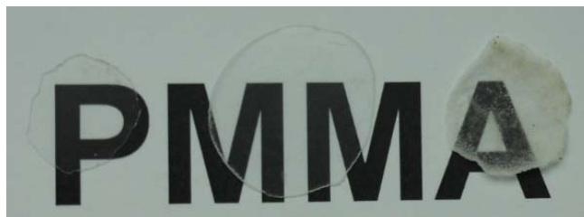
Figure 122. Photograph of hot pressed, 0.25 mm plates of PMMA nanocomposites for UV/VIS measurements, from left to right: blank PMMA, 5 wt% MA-C10-TMS@SiO 2 small, 5 wt% DTMS@SiO 2 small.
