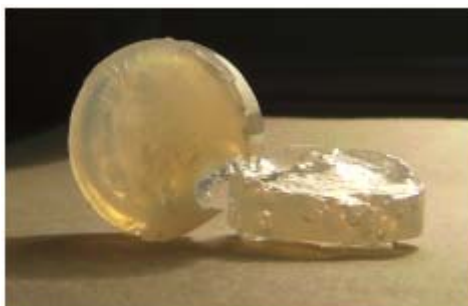
Figure 119. Photograph of PMMA nanocomposites with 5 wt% MA-C10-PA@ZrO 2 large (lying) and 15 wt% MA-C10-PA@ZrO 2 large (standing).
