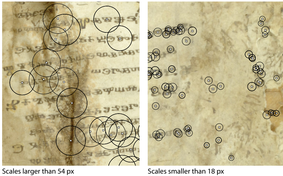
Figure 4.9: Interest points having a scale larger than 54\text{ px} (left), respectively smaller than 18\text{ px} (right). (The resolution of the image considered is 2848 \times 3963\text{ px} )
