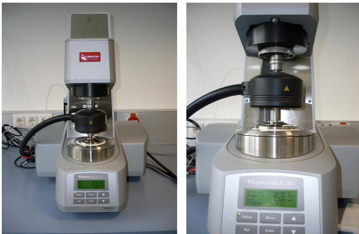
Fig. 10.1: Rheometer with plate-plate measuring system and Peltier hood
