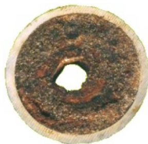
Fig. 6.1: Reduced effective pipe diameter due to wax depositions [7]
