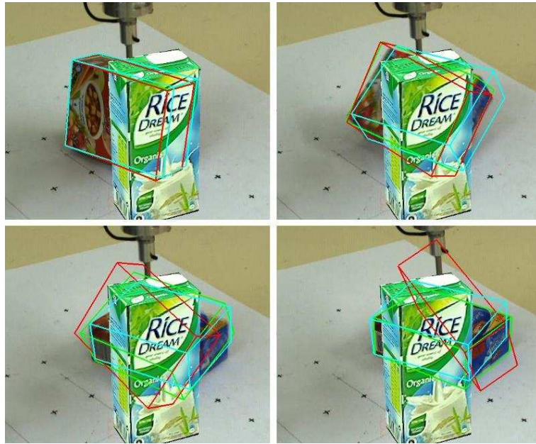
Figure 4.9: The toughest case: toppling combined with occlusion. (colour-based tracking with prediction: green, without prediction: red, pure prediction: blue)
