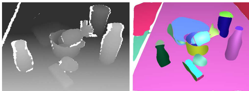
Figure 2.1: Segmentation of an range image captured by sensors such as the Microsoft Kinect. Left: Output of the sensor with missing data points (white). Right: Parametric models like planes and B-spline surfaces trimmed by curves.
