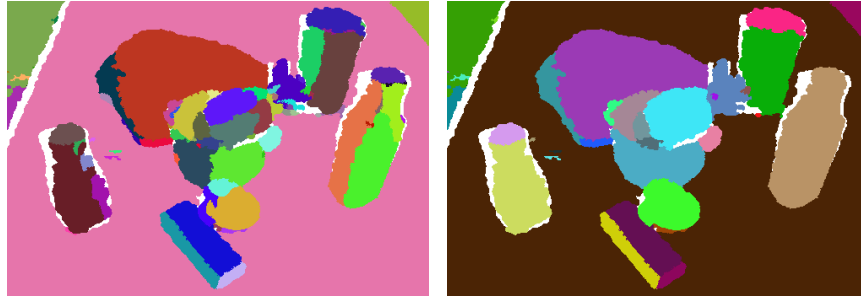
Figure 2.16: Merging planar regions using B-spline surfaces of higher polynomial order.
