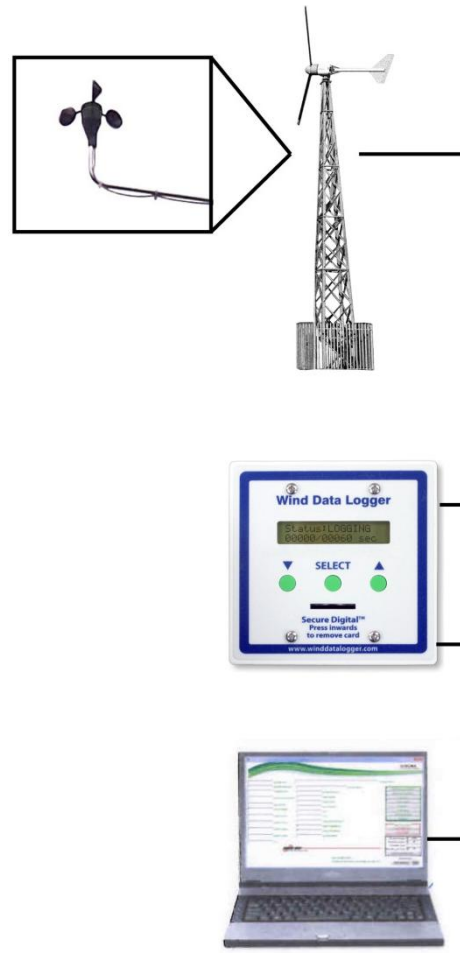
Fig. 3.3.2. Wind data monitoring system, UCC
