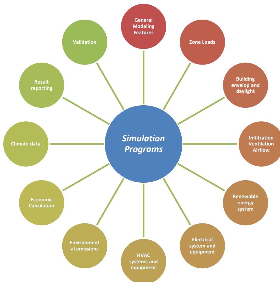
Figure 1.2: Overview of basic building simulation software features (Crawley et al. 2008)
