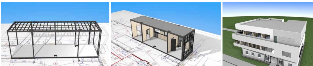
Figure 2.11: Room Module Style scheme (Stugeba 2012)
