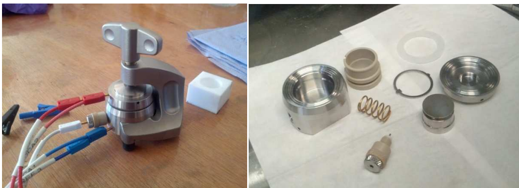
Figure 27: Assembled (left) and disassembled (right) coin cell
