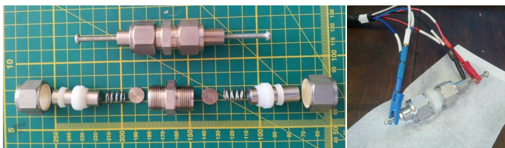
Figure 29: Assembled (left, above), disassembled (left, below) and connected (right) Swagelok cell
