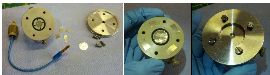
Figure 32: Assembling of the in situ Raman cell from left to right
