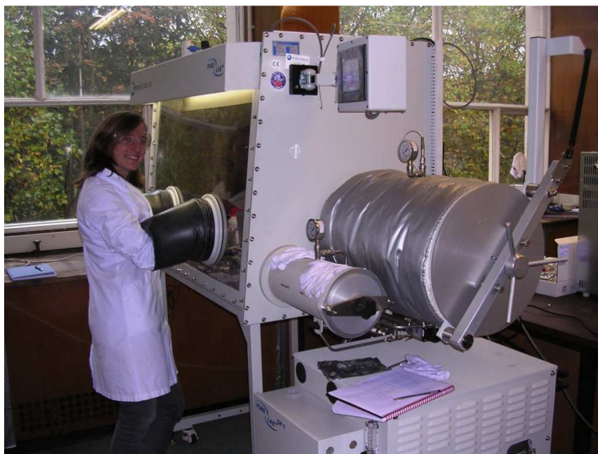
Figure 35: Glove box – Inert Lab 2 GB Glove Box System (IT – Innovative Technology)
