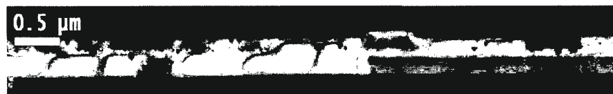
Figure 5.14: TEM cross section image of the seed layer. The long dark grain at the bottom side of the cross section has a (100) surface plane proved by shadow imaging. (This proof is not shown here.)
