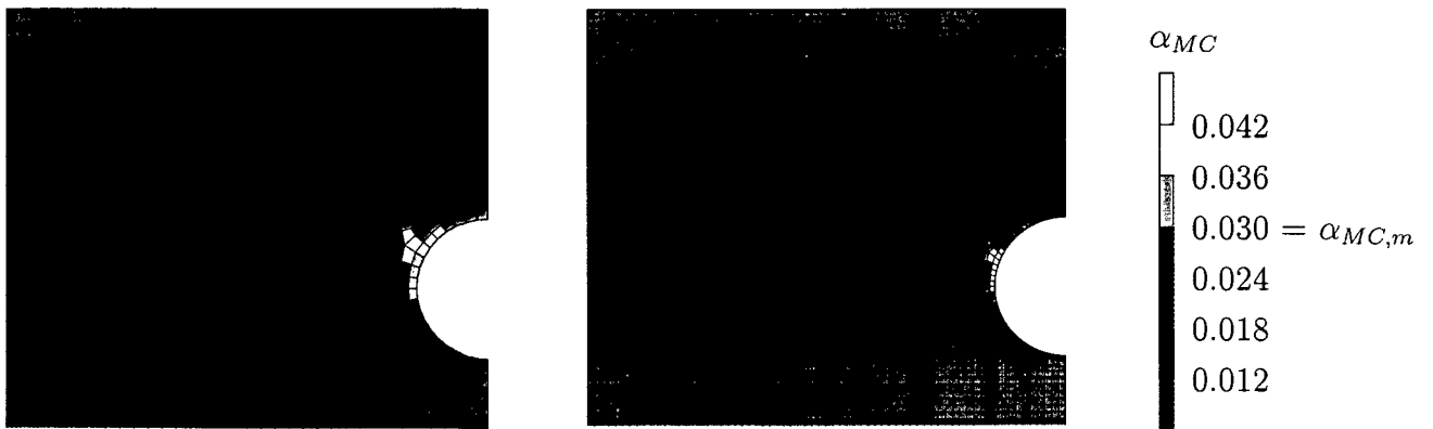
Figure 4.10: Simulation of tunnel excavation: distribution of strain-like internal variable \alpha_{MC} obtained from analysis based on the two meshes, at collapse, i.e., at p/p_0 = 0.04 for mesh 1, respectively at p/p_0 = 0.08 for mesh 2
