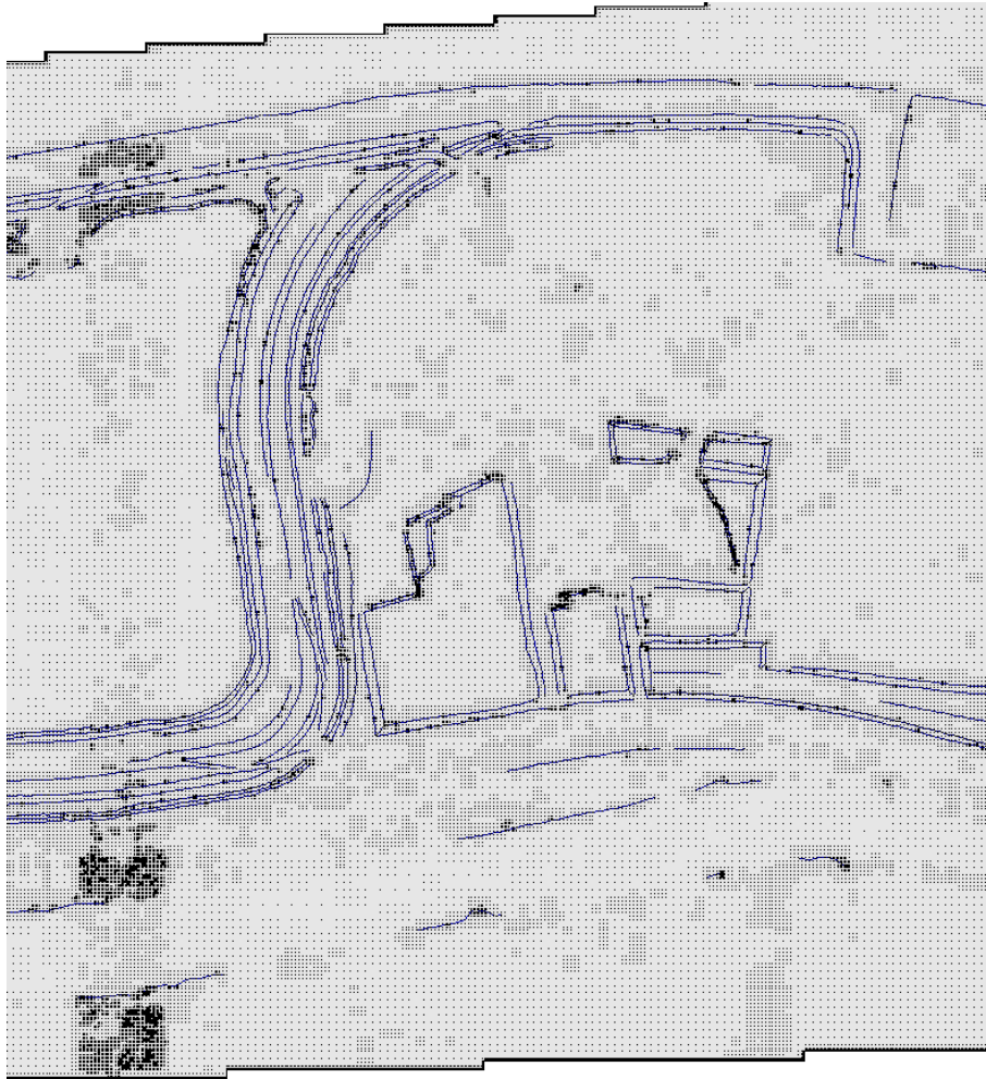
Figure 6.9: Practical example (project area Elbe): Data reduction of a hybrid ALS DTM.
