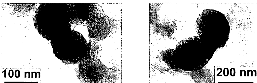
Figure 35: TEM images of TiO 2 particles prepared from a 3-chloro-pentane-2,4-dione containing precursor (diameter of 80 nm) and a 3-acetyl-5-bromo-5-methylhexane-2,4-dione containing precursor (diameter of about 200 nm).
