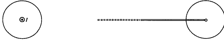
Figure 3.5: Equivalence of a line current (left) and a double-layer of magnetic surface charges (right). Both source configurations yield the same magnetic field outside the support of the source fields.
