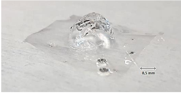
Figure 18: Photographic recording of osmotic deformed Nafion membrane
