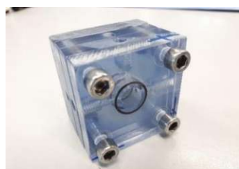
Figure 2: Basic body of the diffusion cell
