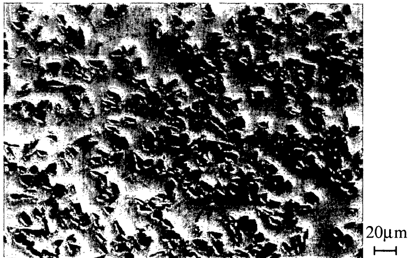
Figure 1.2: Microstructure of a typical aluminum silicon carbide ( \text{Al}/\text{SiC}/20_p ) metal matrix composite material
