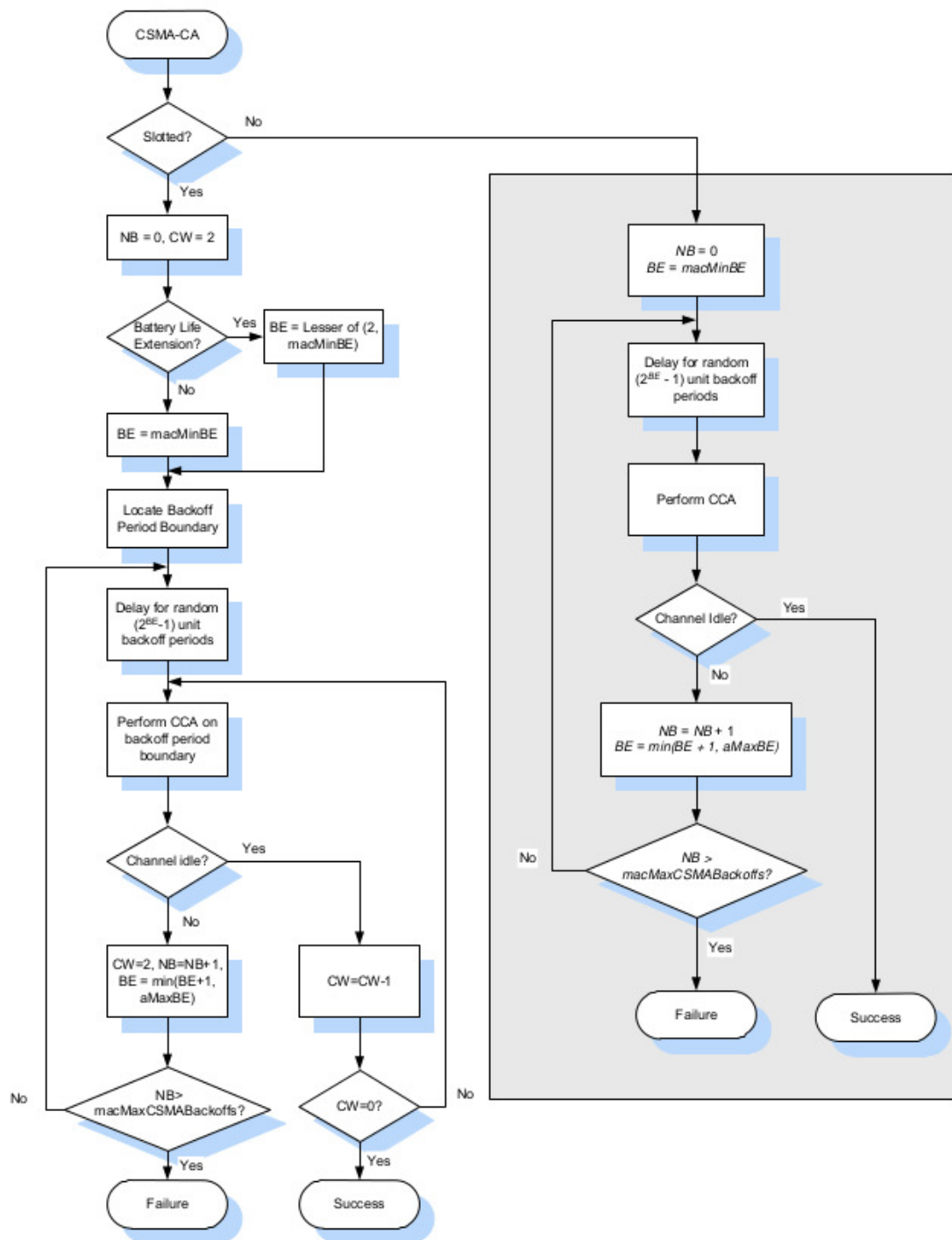
Figure 4.5: CSMA/CA mechanism (with the highlighted unslotted part) [21]
