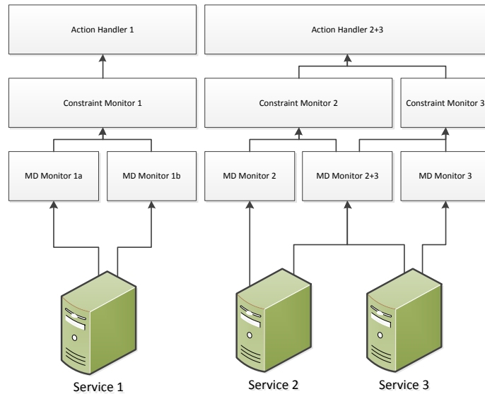
Figure 7.5: Potential Scaling of the Monitor.
