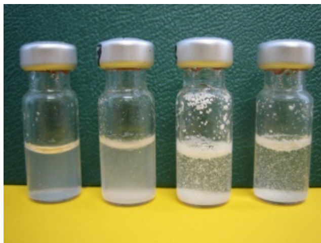
Figure 4.35: Digital image of silica nanoparticle networks with one imidazolium unit with (from left to right) \text{Cl}^- , \text{BF}_4^- , \text{PF}_6^- and \text{Tf}_2\text{N}^- as anion.
