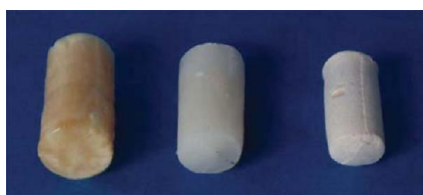
Figure 7.3: Lyocell bodies at different stages of the aerogel production: solidified NMMO melt containing 3% cellulose (left), cellulose gel after regeneration (middle) and supercritically dried cellulose aerogel (right). 203
