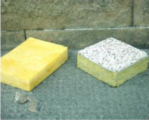
Flexible insulation bat on the left offers greater potential for re-use. Source: F. Stevenson
