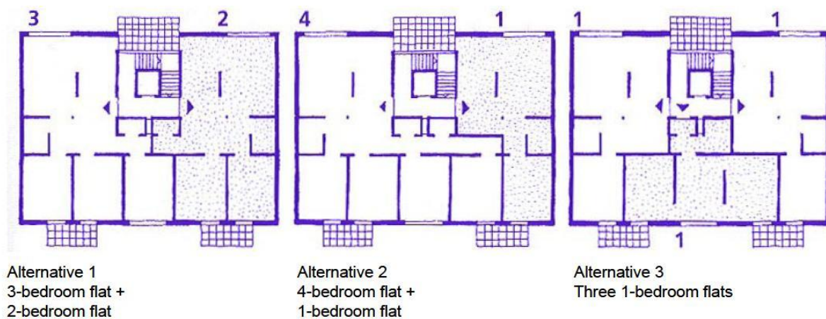
Figure 3.3. Flexibility of the building plan ensures longer life cycle and functional rearrangements (Morgan C., & Stevenson F. 2005 ).
