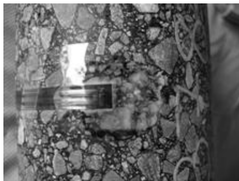
Figure II-10. End of an SG glued to an HMA specimen.
