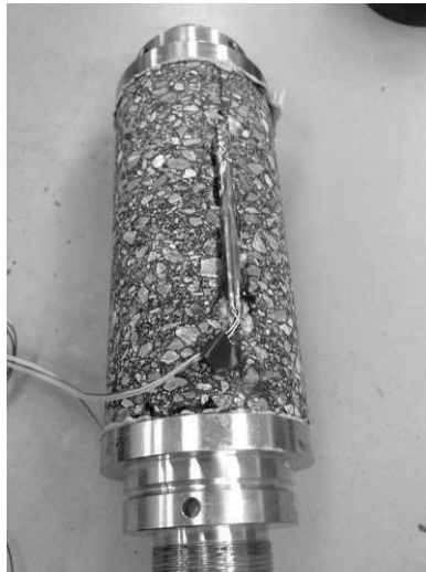
Figure II-14. HMA specimen glued to the load plates with an SG attached on both ends in axial direction.
