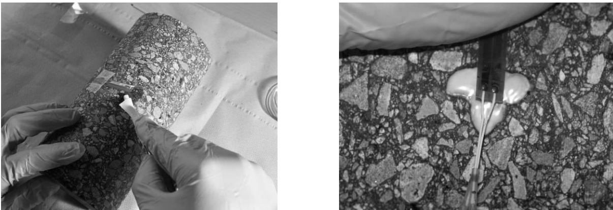
Figure II-11. Cleaning of the adhesive area (left) and attaching the SG to the glued area (right).
