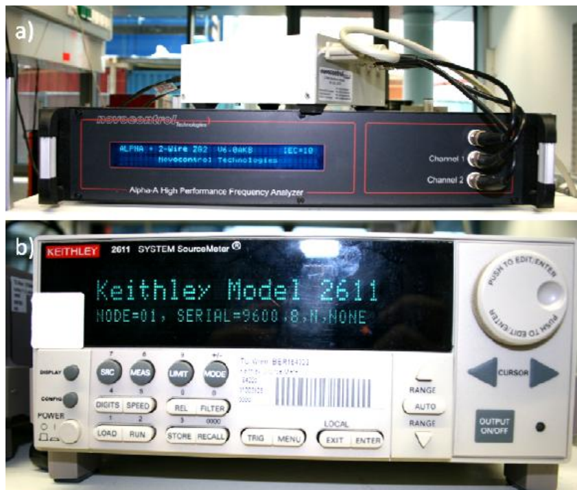
Abb. 6.5: a) Alpha-A high performance frequency analyzer und b) 2611 System SourceMeter Quelle: [37]
