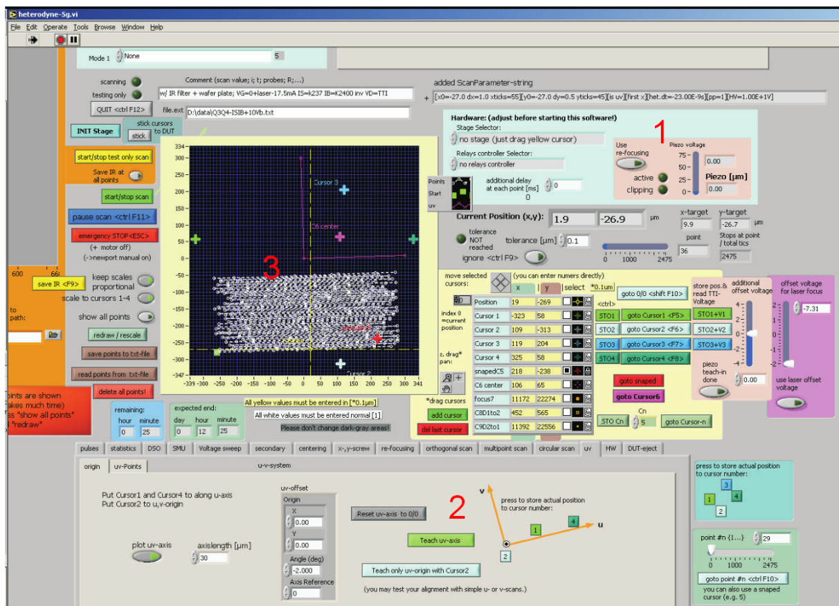
Figure B.2: Screen shot of the heterodyne scanning software heterodyne.vi with re-focusing feature (“1”) and second coordinate system (“2”). To speed up the user interface, several scanning points in the coordinate field (“3”) can be skipped during redraw.
