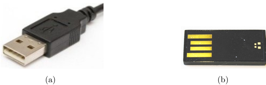
Figure 1.12: USB plug (a) with shield contacting first and (b) longer power and ground pins.
